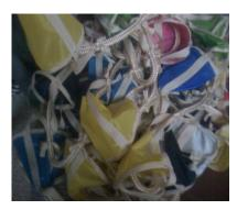
Cones are made from Ripstop Nylon 1.5 oz. cut to the Pattern. You can get approx. 15 cones per 39" wide yard. Several sources on ebay sell for \$3 to \$12 per yard. Many of the yards are 60" or more in width which provide many more cones per yard. I bought an additional 6 yards 60" width for \$38 including shipping.
