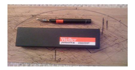
Electric soldering iron if needed, Weller makes many suitable models to be used as a hot knife. Careful to be able to keep the heat low enough so it doesn't smoke and burn. Probably 25-35 Watts is enough. Need a very small tip. These can be found in flea markets or pawn shops for a few dollars. I use one when I need to cut line larger than 5/8"
